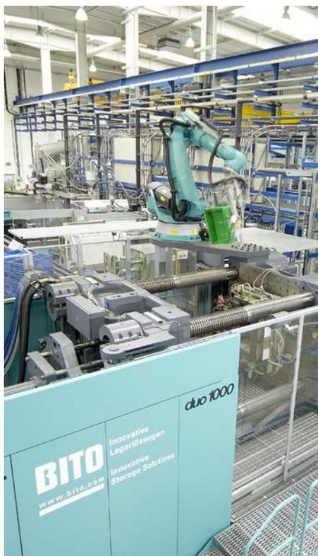
BITO bins and containers are produced in one of the most modern plants of the industry on high performance injection moulding machines with a clamping force of up to 27000 kN. After production, our bins and containers pass through our 600 sqm finishing centre where they are given the final touch to meet customer specific requirements. The entire manufacturing process combines high levels of automation with utmost versatility.
